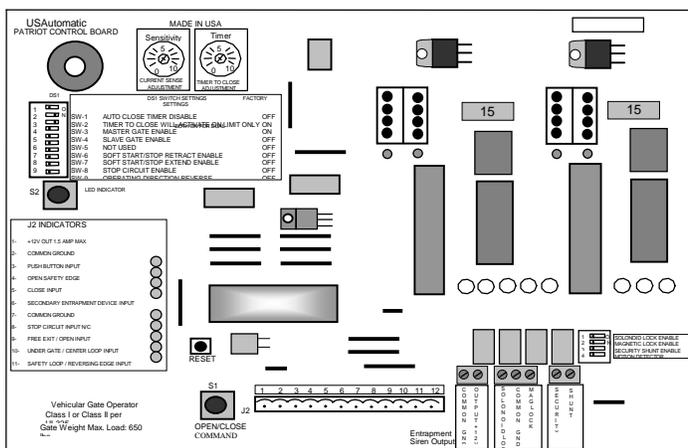
Mag lock and Solenoid lock outputs are labeled On the circuit board. Take care when running wires to avoid pinch areas.
