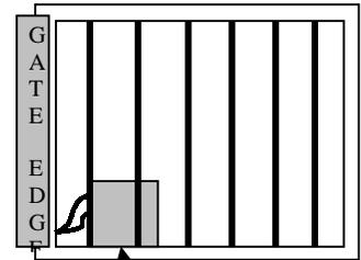
Wireless transmitter connected to gate contact edge.
