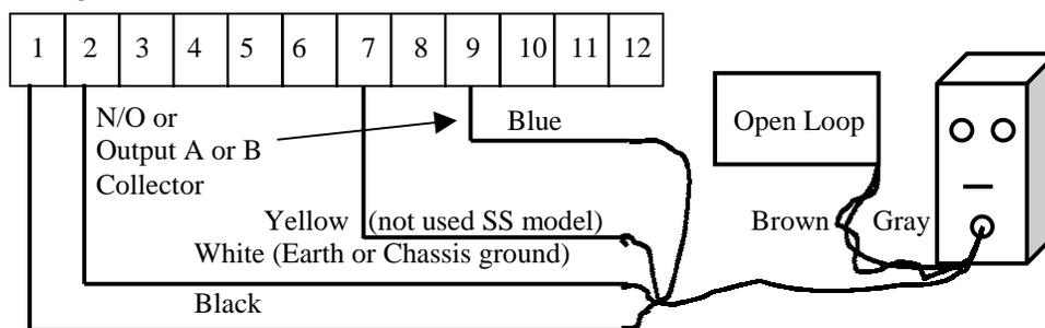
**Wiring Note:** When using the SS model detector connect detector pins 2 (“power –”) 5 and 9 (“Output A, B Emitter”) Together.
