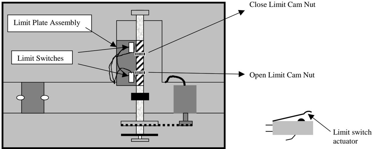
**NOTE:** *DO NOT ADJUST THE LIMIT CAM NUTS PAST THE LIMIT SWITCH ACTUATOR ARM. THIS MAY RESULT IN DAMAGE TO THE LIMIT SWITCH. ENSURE THE LIMIT PLATE ASSEMBLY SNAPS INTO THE GROOVES ON THE LIMIT ADJUSTMENT CAMS PRIOR TO OPERATION.*
