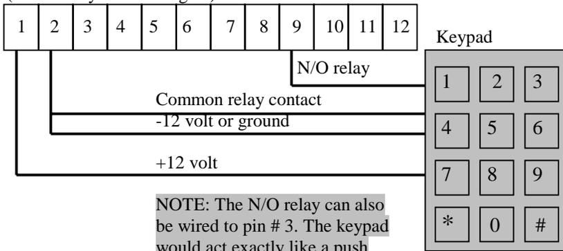
NOTE: The N/O relay can also be wired to pin # 3. The keypad would act exactly like a push button transmitter when code was entered. Maintain open pin # 9.
