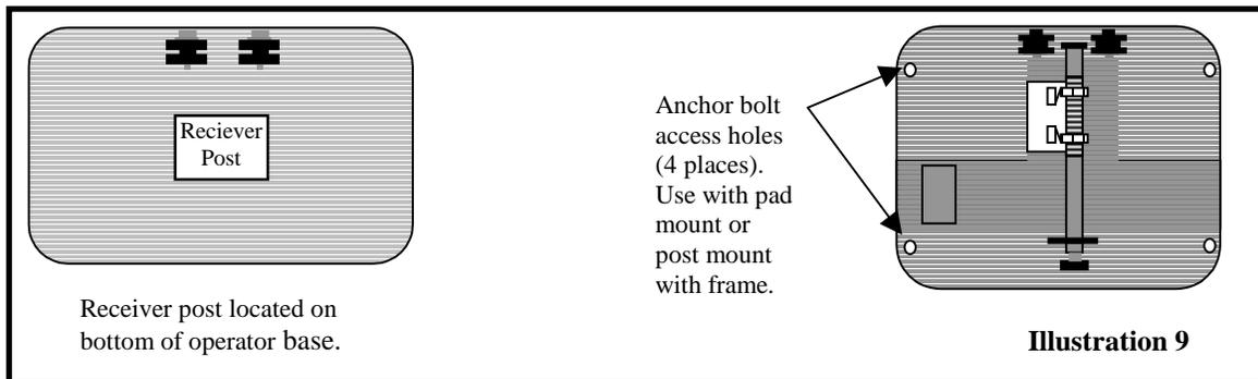
**NOTE: Regardless of mounting method ensure that operator base does not extend into the driveway area, where damage from traffic could occur.**
