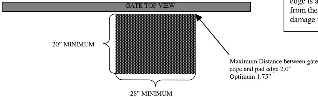
When determining pad location ensure that the operator's outer edge is a safe distance away from the driveway to avoid damage from traffic.
