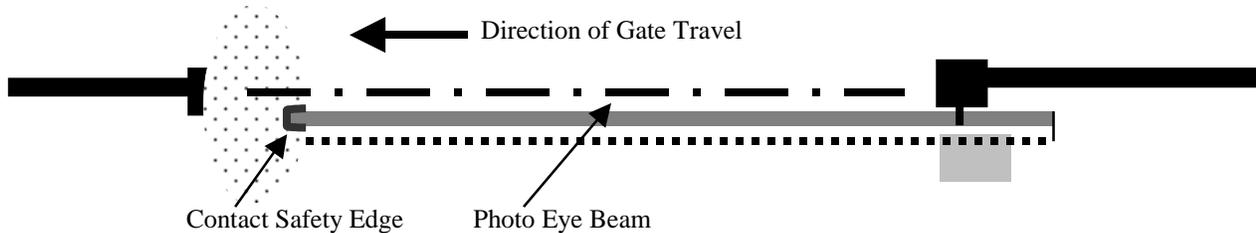
**Zone 2** A safety edge may also be utilized here but the best remedy is to eliminate pinch points when designing the gate. Most injuries at this point result from negligence, such as reaching through the gate to activate a button, key switch, etc., or riding the gate open.
