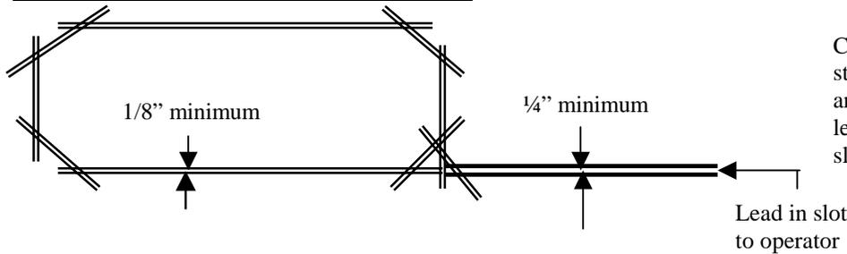
Corners should be cross-cut as shown for stress relief. 45 degrees is maximum turn angle allowed. Sawcut width must be at least 1/8" for recommended wire. Lead in slot must be at least 1/4" for twisted leads.
