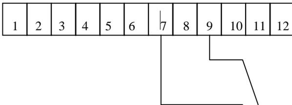
Normally open contacts from any device such as a Free Exit Loop, Maintain Contact Key switch, 7-Day Timer, Telephone Access Unit etc. When the switch contacts close, the gate will open and remain open until the contacts are released. The Close Timer or any close signal will only operate after the switch contacts open.
