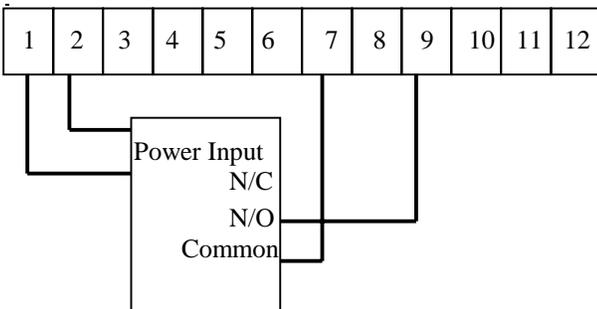
**NOTE:** This type of detector senses moving vehicles only. It should be utilized as an opening device only. If used as a safety device, the gate will close if the vehicle stops and possible damage will result.
