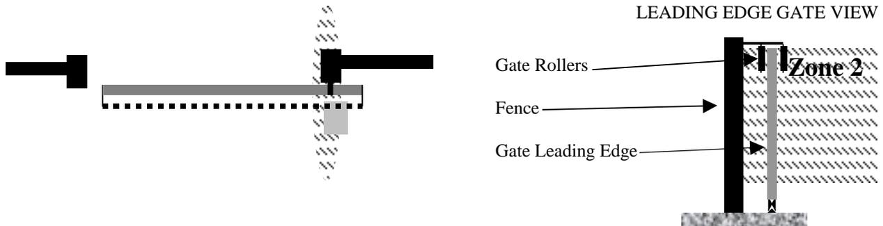
**Zone 3** This area is best protected with proper gate construction and installation. Care must be taken to minimize the exposed wheel to track area. A photo-eye or contact edge might also work in this area depending on your gate construction.
