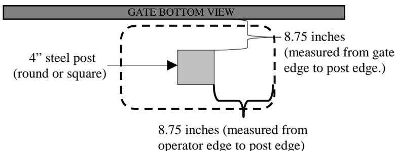
When determining post location ensure that the operator's outer edge is a safe distance away from the drive to avoid damage from traffic. See illustration 13 for operator base overall dimensions.
