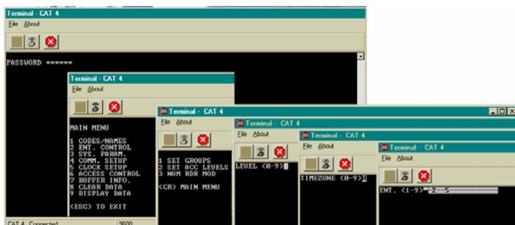
Access Levels are used to attach Time Zones to specific Entrances. Only one Time Zone is allowed per Access Level. Any combination of entrances may be selected, but at least one entrance must be selected, or the affected Access Level will not function. From one to four entrances may be assigned
