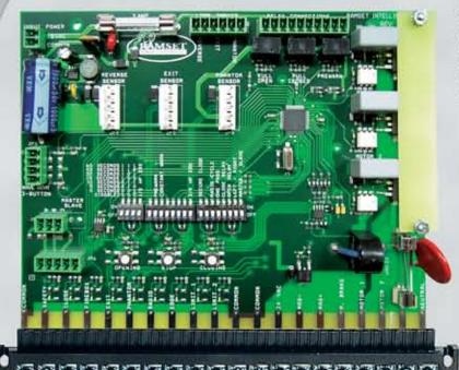
I he Intelligate control board is the most advanced gate controller in the industry, putting Ramset ahead of the competition when it comes to reliability and number of features. It is controlled by a programmable microprocessor that reads and precisely executes all functions of the control board. Some of the features of the control board
