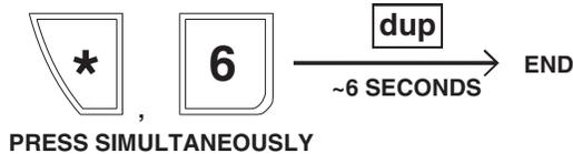
**Note:** To duplicate memory, plug backup memory module into backup slot and press **\*6**. Once duplication is complete, remove the backup memory module and store in a separate location.
