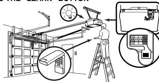
1. Press and release the "learn" button on motor unit. The learn indicator light will glow steadily for 30 seconds.
