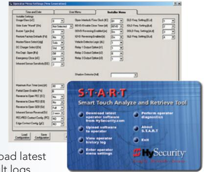
Smart Touch Analyze and Retrieve Tool allows users to upload latest operator software, download fault logs, generate diagnostics, and program the operator using a laptop.
