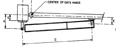
Figure 4. Important mounting dimensions for inward swing 400 operators, top view
