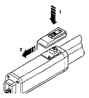
Figure 8. Install the locking cap cover
