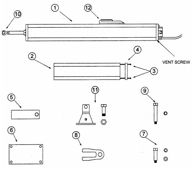
Figure 1. Parts of the 400 Operator
