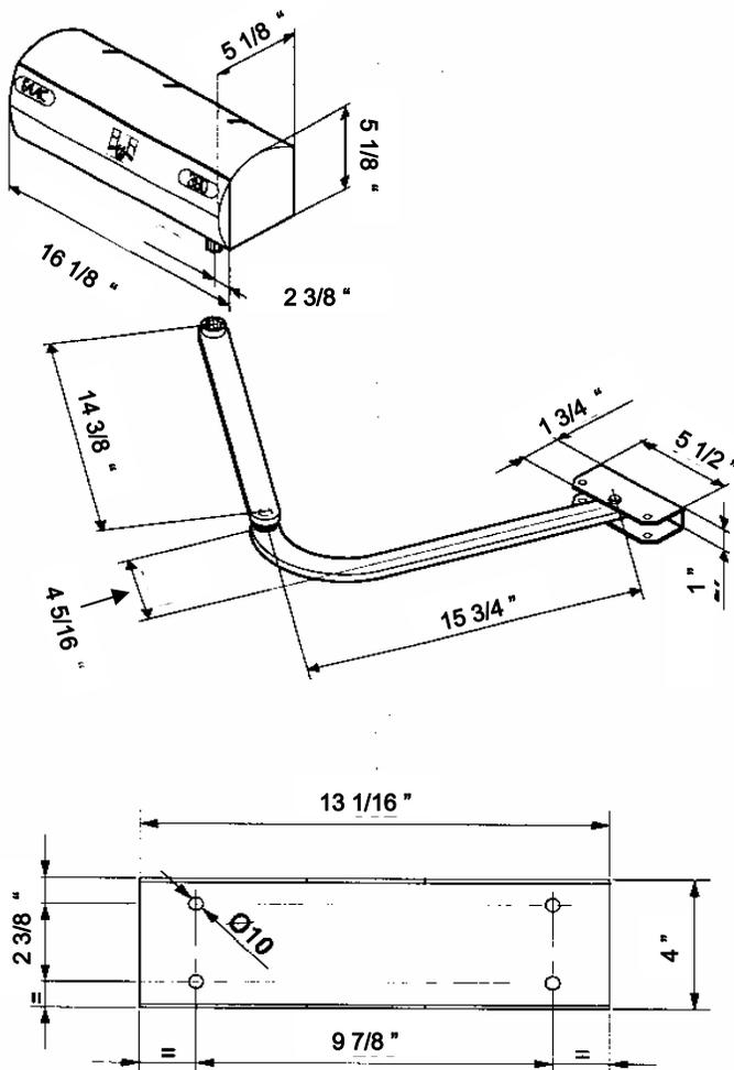
Figure 1. 390 Operator Dimensions
