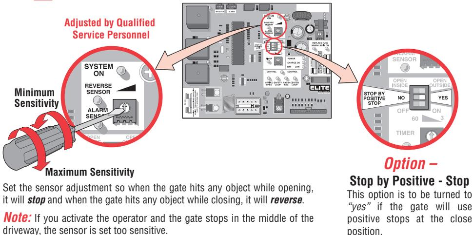
**Important:** It is necessary to still adjust your limit switch at the close position. The controller will look for the limit close first and then it will look for the positive stop.
