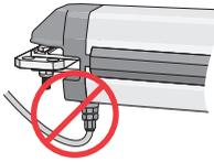
**Caution:** Do **Not** over-bend the cord from the operator. Doing this will cause the wires to eventually break.
