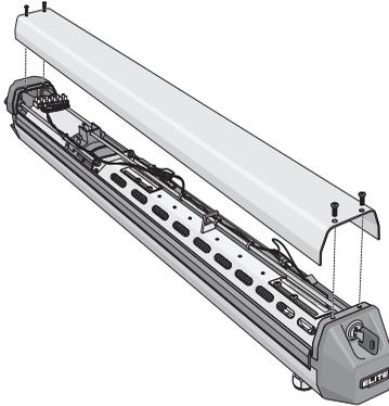
**Step 2:** Release the mechanical lock by turning the key to the horizontal position.
