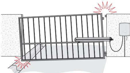
③ Gate hinges are too tight or broken and the gate is not moving freely.
