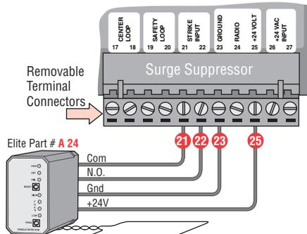
Allows gate to automatically open for exiting vehicles.
