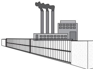
**Commercial/General access vehicular gate operator – Class III** – A vehicular gate operator (or system) intended for use in an industrial location or building such as a factory or loading dock area or other locations not intended to service the general public.
