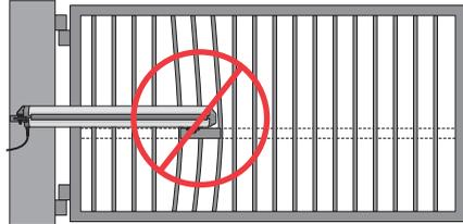
**DO NOT** install on a few pickets, they will bend. Weld a reinforcement bar across entire gate.
