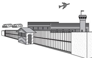
**Restricted access vehicular gate operator – Class IV** – A vehicular gate operator (or system) intended for use in a guarded industrial location or building such as an airport security area or other restricted access locations not servicing the general public, in which unauthorized access is prevented via supervision by security personnel.
