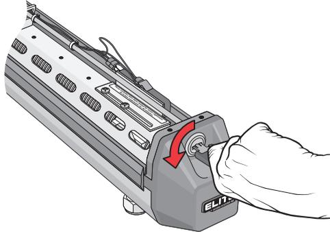
**Step 3:** Position the Miracle 1 *horizontally level* on the closed gate, where desired. For strength purposes, the front steel bracket *must* be attached in an area that can withstand *heavy forces*. Additional reinforcement steel plates may be necessary for mounting.
