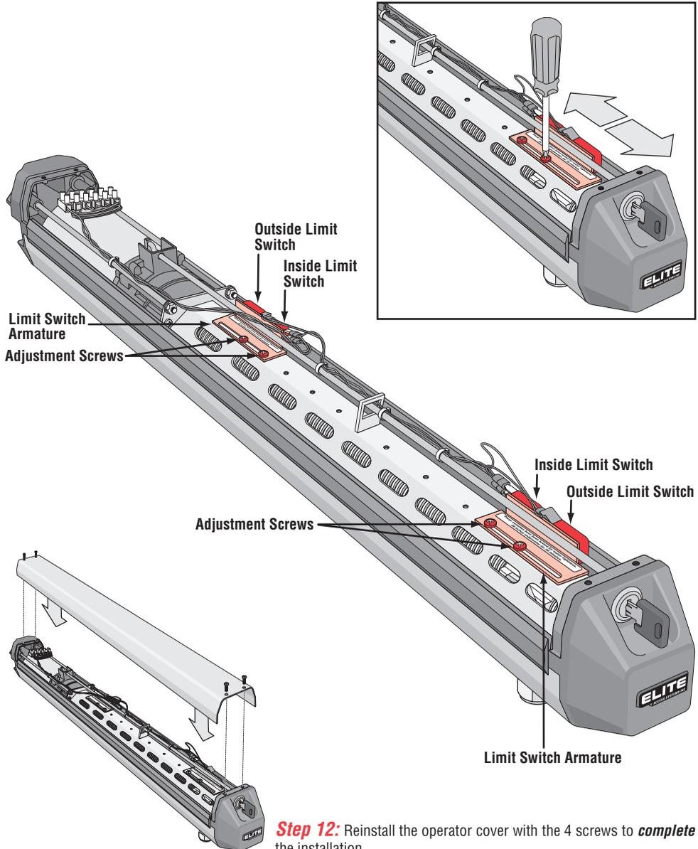
**Step 12:** Reinstall the operator cover with the 4 screws to **complete** the installation.
