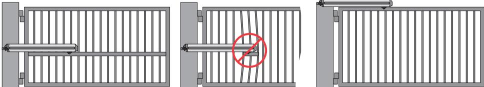
If using a gate crossbar, weld bar across *all* pickets. **Do not** weld the crossbar on a few pickets, or they will bend.
