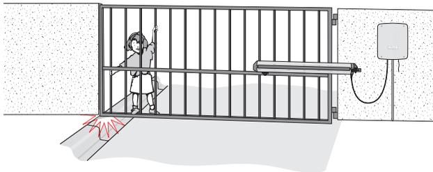
② A foreign object is on the gate frame while the gate is moving.
