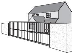
**Residential vehicular gate operator – Class I** – A vehicular gate operator (or system) intended for use in a home of one-to four single family dwelling, or a garage or parking area associated therewith.
