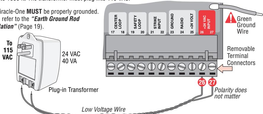
**!** **Caution:** Use low voltage direct burial landscape lighting cable – 14 gauge/300 watt not exceeding 500 ft. For longer than 500 ft, use 10 AWG wire up to 1000 ft.
