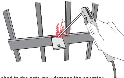
**Caution:** Welding the brackets with the operator attached to the gate may damage the operator.
