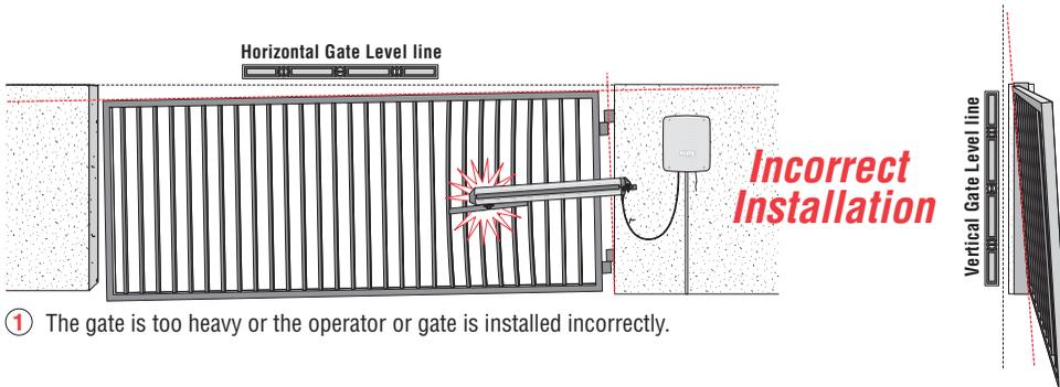
① The gate is too heavy or the operator or gate is installed incorrectly.
