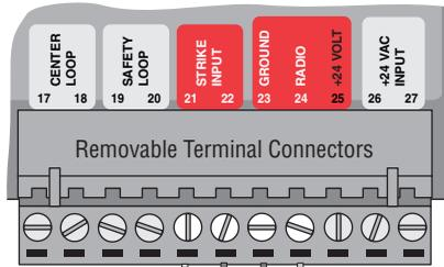
**Caution:** Make sure **BARE WIRE** makes good contact inside removable terminal connectors. **DO NOT** let wire insulation interfere with connection.
