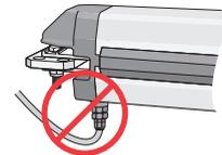
**DO NOT** over-bend the cord from the operator. Doing this will cause the wires to eventually break.
