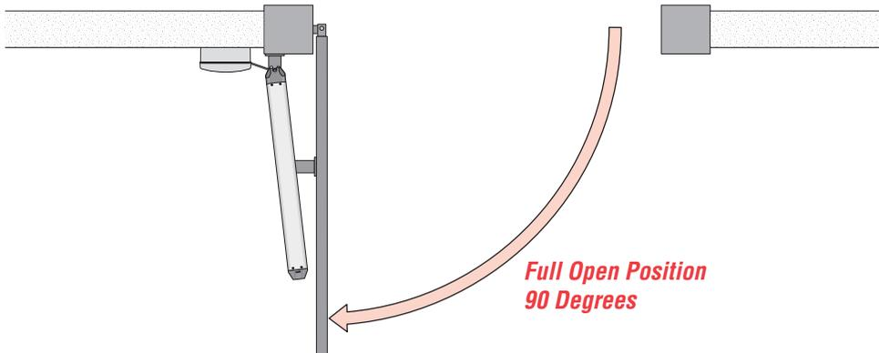
**Step 3: Re-Lock** the operator by turning the key clockwise while pushing or pulling on the gate until you hear the key release click into place. The operator can resume normal operation as soon as power is restored.
