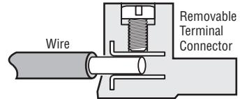
**Caution:** Make sure **BARE WIRE** makes good contact inside removable terminal connectors. **DO NOT** let wire insulation interfere with connection.
