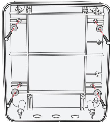
Mount control box with four screws and washers (recommend #10 thru 1/4-20 Bolts or Screws) **Do Not** over tighten.
