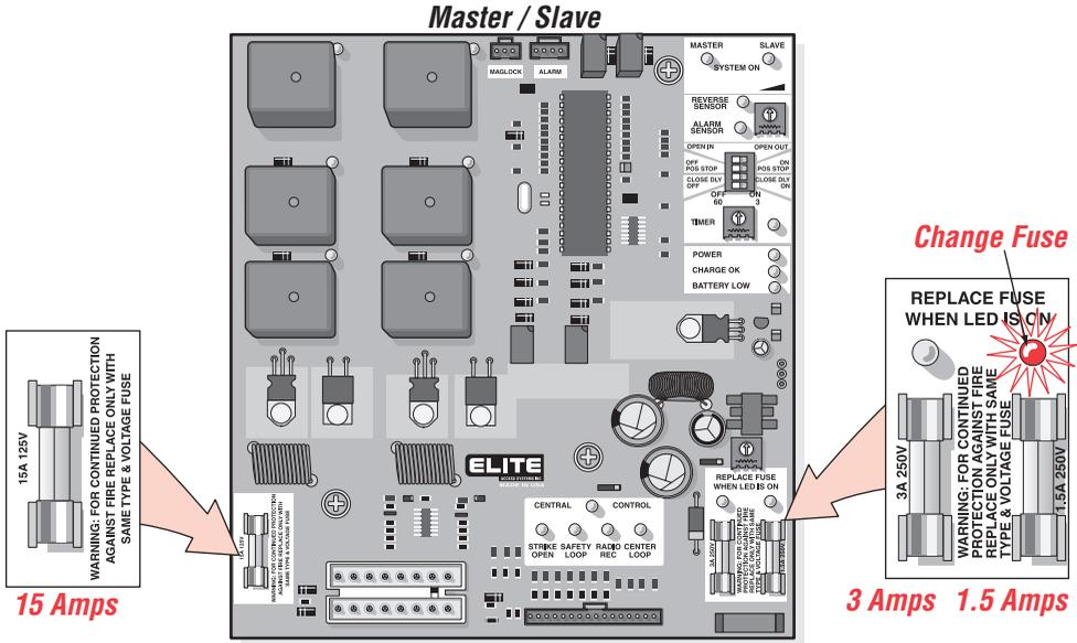
**⚠ Caution:** If left side board fuse is blowing on a regular basis, make sure operator is operating smoothly. Verify traveler carriage washer placement (Page 12). Check motor wire connections. Replace the fuses only with specified rating (Supplied by Chamberlain Elite).
