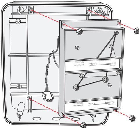
Remove the four nuts and remove battery rack. Reverse this process to reinstall.
