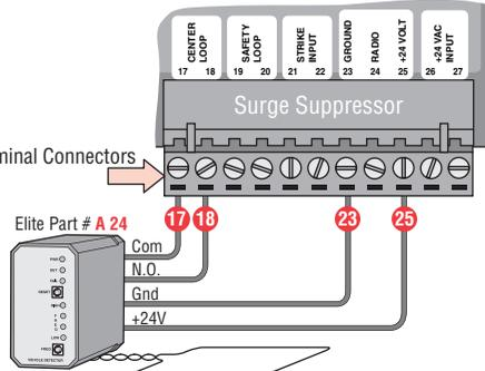
For fail safe operation, connect safety loops in series.
