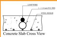
Ty-Wrap 1-1/4' PVC pipe to the top of the rebar in the size and loop to the top of the PVC frame. This stabilizes the loop during the
