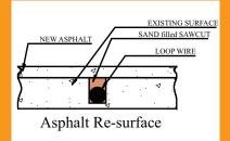
Saw cut existing surface 3/4" deep and place loop into bottom of saw cut. Place sand over loop wire to surface of existing surface and
