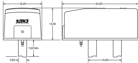
Post mount operator Height is adjustable by the installer.
