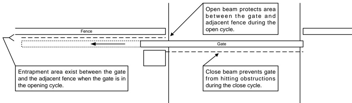
For gate operators utilizing a contact sensor:
