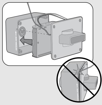
Insert battery pack facing away from circuit board and attach cover.
