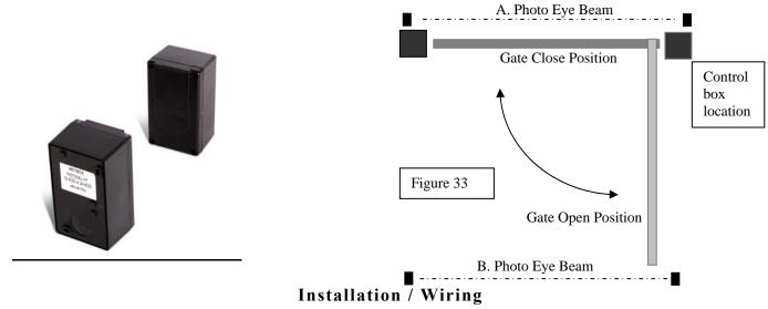
Select a proper installation site, where the transmitter and the receiver can be along the same line and at the same height. Remove the cover from both units. Attach back plate to the installation site using mounting holes in back plate.
