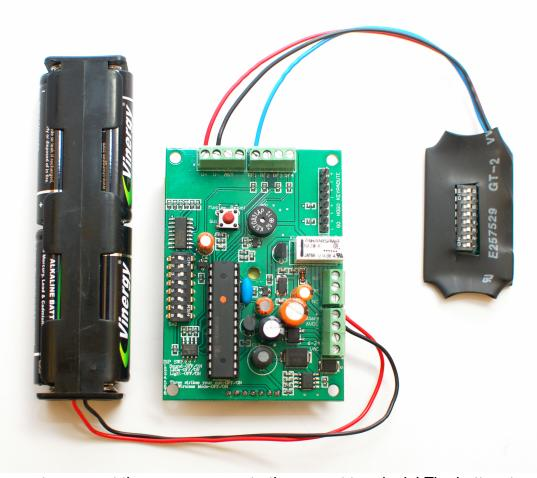
• **NOTE:** Be sure to connect the power source to the correct terminals! The battery terminals and the AC/DC terminals are different.
