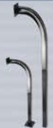
Goose Necks Square - 14 ga. Available in 48" padmount or 66" in-ground. Used for mounting keypads, phone entry systems, card readers...etc.
