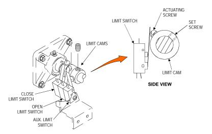
Note: Limits are set for 90 degree arm movement at factory.
