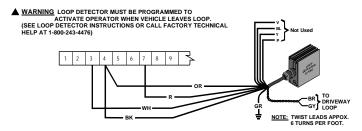
4. The **Quick Close Loop** (Anti-Tailgate feature) is usually used for one way traffic. It can only be activated when there is no input from an "Open" or "Close Safety" device. Once activated it will disable any "Close Safety" device and can only be overridden by an "Open" input. Therefore, this option should only be used in secure applications and a close warning device should be connected to terminals W1 and W2. (See "Close Warning Connection Diagram")
