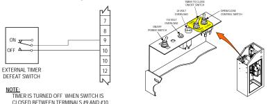
2. Move the "Timer To Close" switch on the operator control panel to the "ON" position.
