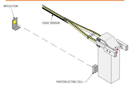
NOTE: 24 VAC power is available between terminals 3 & 4 for devices such as photo eyes, wireless edges, etc. All safety device contacts must be NORMALLY OPEN.
