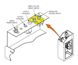
The **AUTO RECLOSE TIMER** adjustment screw is located on the printed circuit board. The operator is shipped from the factory with this timer preset to the "MIN." position; fully counter clockwise, and the "TIMER TO CLOSE" toggle switch in the "OFF" position. As the timer adjustment screw is rotated clockwise, the closing of the gate can be delayed from 1 second to 10 seconds.
