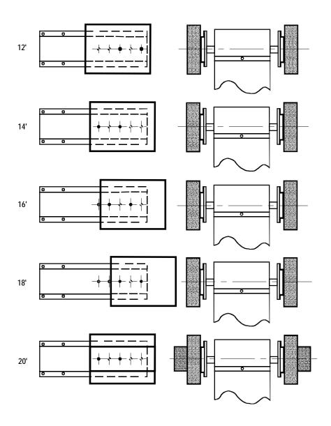
3. Adjust arms to the desired horizontal position, equal in height and secure by tightening the 1/2" mounting hardware.
