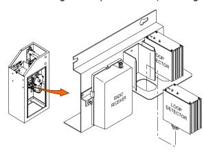
8. Connect loop detector to the control board and the wire loop as shown in the following diagrams.
