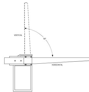
1. In order to achieve 90 degree arm movement from the drive linkage, the limit cams must be set to obtain the linkage positions shown below.
