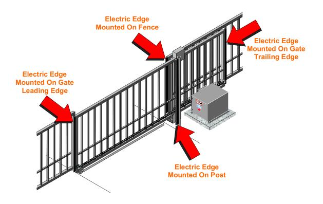
2. Connect contact sensor edges to the control board as shown in the illustration below. CONTACT SENSOR CONNECTION
