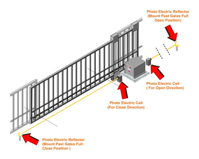
3. Connect **NON-CONTACT** sensors to the control board as shown below.
