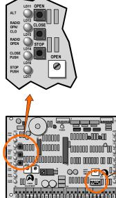
**NOTE:** If Dipswitch #3 is in the "**ON**" position for use with a **NORMALLY CLOSED** "**STOP**" **BUTTON**, then the board mounted "STOP" button must be held depressed in order to use the open and close buttons. Releasing the stop button will then stop the operator.
