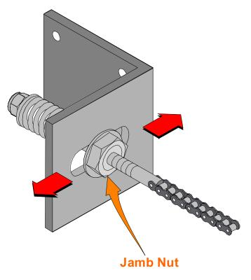
11. Adjust chain tension so that the chain tension springs are reduced to a length within 1-7/8" and 1-3/4".
