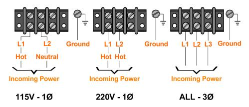
**NOTE:** Wiring to operator must use watertight materials in accordance with local electric code. See wire gauge/distance charts for proper sizing. Master/Slave installations should have **SEPARATE** power supply wiring or length of wire runs should be figured at half that shown on the chart. **This unit must be grounded in accordance with N.E.C. and local codes.**
