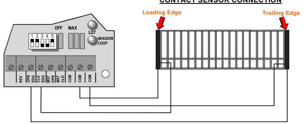
**<u>NOTE</u>**: Leading edge is connected to "**CLO EDG**" and "**COM**" terminals. Trailing edge, Post Mounted edge and Fence Mounted edge are connected to "**OPN EDG**" and "**COM**" terminals.
