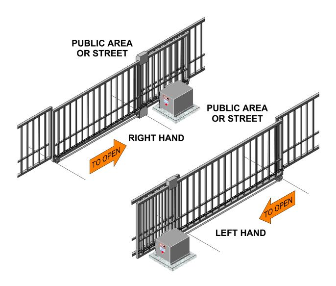
**NOTE:** This unit is factory setup for **<u>RIGHT HAND</u>** operation. To convert operator to left hand operation move dipswitch #2 to on position.
