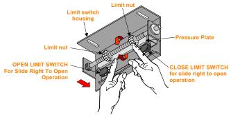
16. After the desired open and close position of the gate has been obtained, make certain that a groove in both limit nuts are engaged by the pressure plate.
