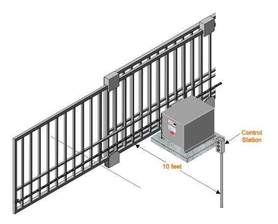
▲ 6. Attach large warning signs provided to each side of gate in the most conspicuous place. Mount control station and smaller warning placard together within sight of the gate opening.
