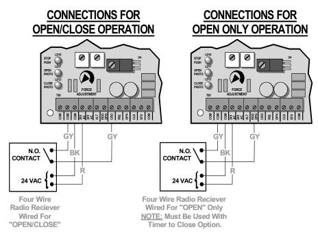
1. For electrical connections of a four-wire radio receiver via the external terminal strip. See below.
