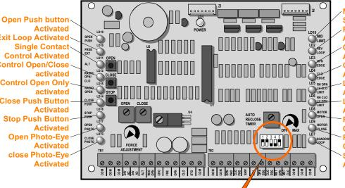
**Mid-Stop Limit** Switch Activated **Reversing Loop** Activated **Open Safety Edge** Activated **Close Safety Edge** Activated Limit Switch Activated Limit Switch Activated **Power to Open Contactor coil Power to Close Contactor coil Shadow Loop** Activated
