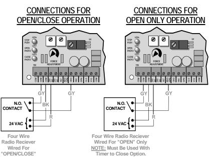
1. For electrical connections of a four-wire radio receiver via the external terminal strip. See below.
