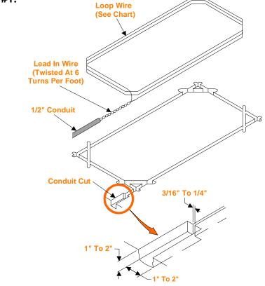
3. Leaving enough wire for the **LEAD IN**, insert the specified number of turns of wire in the cut grooves. (See chart).
