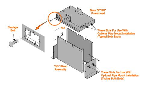
2. Using ½" hardware (Not Supplied) bolt assembled unit to the pad, being sure to align operator parallel to the fence.
