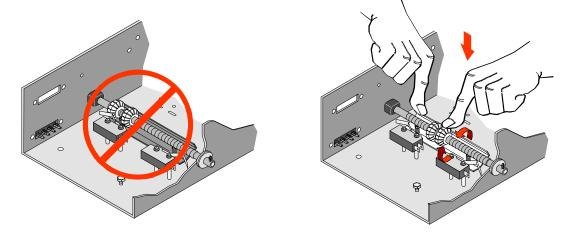
2. With the gate at mid travel, depress the pressure plate and set the grooved limit nuts approximately 1 inch from the limit switches on each side.
