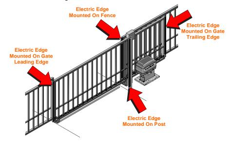
2. Connect contact sensor edges to the control board as shown in the illustration below.
