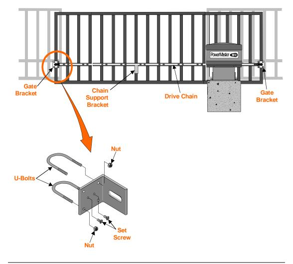
**NOTE:** By moving the gate manually to each end of its travel, chain alignment is simplified.
