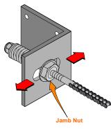
11. Adjust chain tension so that the chain tension springs are reduced to a length within 1-7/8" and 1-3/4".
