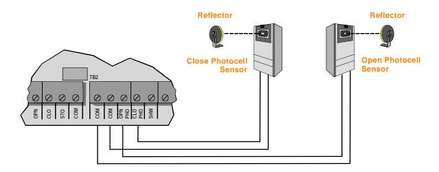
**NOTE:** Close photocell is connected to "CLO PHO" and "COM" terminals. Open photocell is connected to "OPN PHO" and "COM" terminals.
