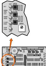
**NOTE:** If Dipswitch #3 is in the "**ON**" position for use with a **NORMALLY CLOSED** "**STOP**" **BUTTON,** then the board mounted "STOP" button must be held depressed in order to use the open and close buttons. Releasing the stop button will then stop the operator.
