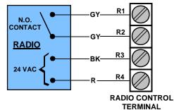
**NOTE:** Internal wiring for the radio control terminal strip is factory set-up for the OPEN ONLY option. For the OPEN/CLOSE option, move the wire on the control board terminal strip from the "RDO OPN" terminal to the 'CRO" terminal.
