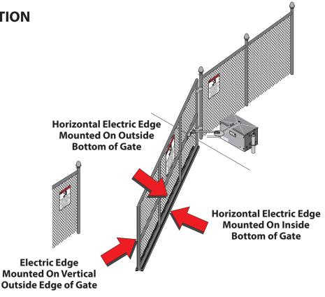
1. Install electric edge sensors in locations shown on the right.
