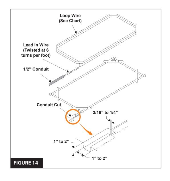
3. Leaving enough wire for the lead-in, insert the specified number of turns of wire in the cut grooves (See chart).
