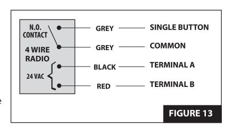
**NOTE:** If your radio's connecting wires are not color coded as shown, see the radio's installation manual to determine which wires are for the normally open contacts and which require the 24VAC Power Supply.
