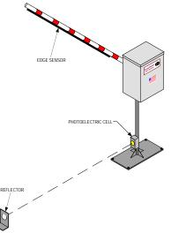
2. Electrically connect sensing system to operator terminal strip as shown  $\neg / \neg$  below.
