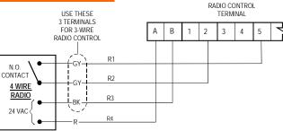
**NOTE:** The radio connections shown above are for "OPEN ONLY" operation. Therefore the "TIMER TO CLOSE" option must be activated for closing. (See next section.) If alternate "Open" - "Close" operation is desired move wire on terminal strip from terminal #2 to terminal #1.
