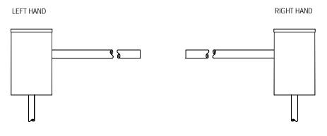
Note: Operators are wired for Right Hand operation at the factory.
