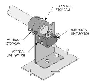
3. Rotate the Arm to the straight up, vertical position. Loosen the set screw on the vertical stop cam and rotate the cam, (clockwise for a **Right Hand** installation and counterclockwise for a **Left Hand** installation) until it just actuates the vertical limit switch. (See diagram.) Secure this position by tightening set screw.
