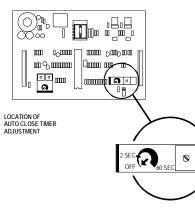
The operator is equipped with a timer to close option for use with **OPEN ONLY** control devices such as a radio control, or card key control. The **AUTO RECLOSE TIMER** adjustment screw is located on the printed circuit board. The operator is shipped from the factory with this timer preset to the off position; fully counter clockwise. As the timer adjustment screw is rotated
