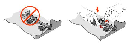
2. With the gate at mid travel, depress the pressure plate and set the grooved limit nuts approximately 1 inch from the limit switches on each side.
