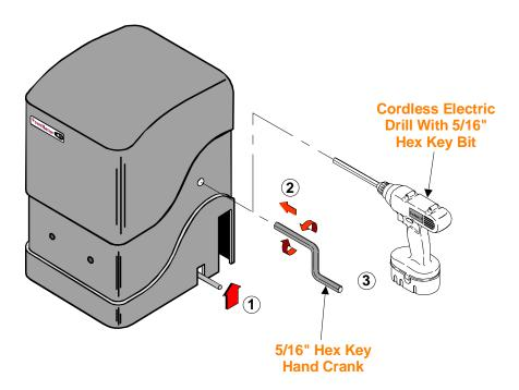
3. Rotate hand crank or use cordless drill to manually move gate in the desired direction.
