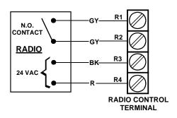
**NOTE:** Internal wiring for the radio control terminal strip is factory set-up for the OPEN ONLY option. For the OPEN/CLOSE option, move the wire on the control board terminal strip from the "RDO OPN" terminal to the 'CRO" terminal.
