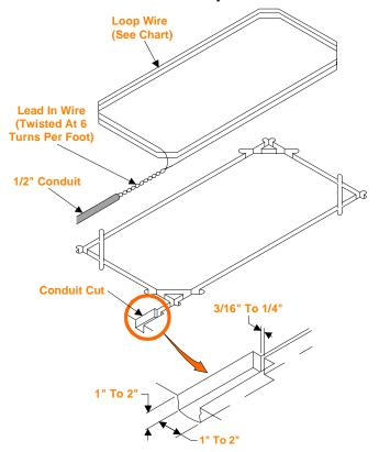
3. Leaving enough wire for the **LEAD IN**, insert the specified number of turns of wire in the cut grooves. (See chart).
