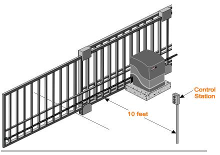
▲ 6. Attach large warning signs provided to each side of gate in the most conspicuous place. Mount control station and smaller warning placard together within sight of the gate opening.
