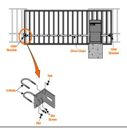
12. Align drive chain to the drive sprocket and ensure it is parallel to gate using slots in gate bracket as shown below.
