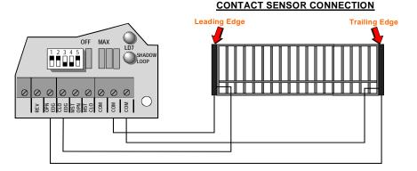
NOTE: Leading edge is connected to "CLO EDG" and "COM" terminals. Trailing edge, Post Mounted edge and Fence Mounted edge are connected to "OPN EDG" and "COM" terminals.
