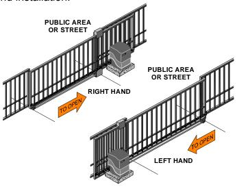
**NOTE:** This unit is factory setup for **RIGHT HAND** operation. To convert operator to left hand operation move dipswitch #2 to "ON" position.
