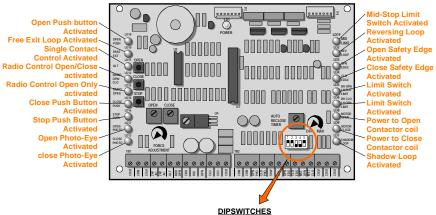
S1 - OFF = NORMAL OPEN/CLOSE PB ON = <u>SAFETY/SECURE</u> MODE
