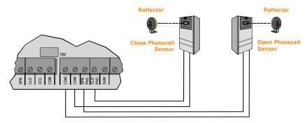
NOTE: Close photocell is connected to "CLO PHO" and "COM" terminals. Open photocell is connected to "OPN PHO" and "COM" terminals.
