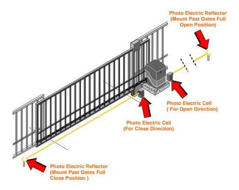
Connect NON-CONTACT sensors to the control board as shown below.
