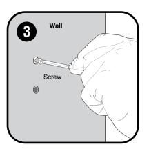
Install mounting screws, allowing 1/8" (3.2 mm) to protrude above surface.
