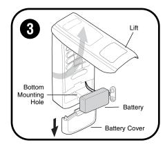
Remove battery cover and battery. Determine location for keypad. Mark the bottom mounting hole.
