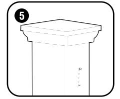
Install top mounting screw, allowing 1/8" (3.2 mm) to protrude above surface. Position keypad on screw head and adjust for snug fit.
