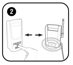
Remove foam spacer on underside of keypad cover. Check range before installing. Using two people, hold the keypad and receiver in the desired locations. Make sure the keypad rings the gatebell when pressed. If no chime is heard, repeat test using a new location for the receiver.
