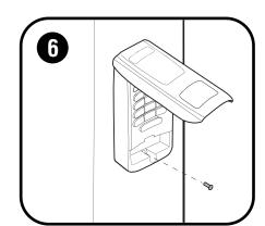
Secure keypad with bottom screw, using care to avoid cracking plastic housing. Reinstall battery and slide battery cover up and snap it into place. Close cover.
