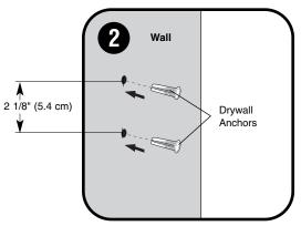
Mark and drill pilot holes using 1/4" drill bit.
