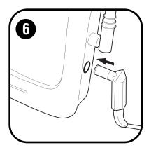
Plug power adapter into receiver. Plug into outlet.
