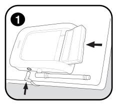
Insert remote control and power adapter into receiver. Plug into outlet.
