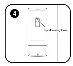
For the top mounting screw, mark 4 1/4" (10.8 cm) up the centerline from the bottom of the keypad. Drill 1/8" pilot holes for top and bottom screws. See keypad mounting reference.
