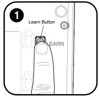
Press and release the learn button on the back of the indoor receiver.
