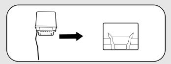
To clear the memory on the OTIU, dial "\*\*#8" on the telephone connected to the OTIU. A beep will be heard.
