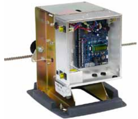
SlideSmart DC - Polyurethane cover removed to expose Smart DC Controller with full 32 character LCD screen and 5 tact buttons for programming; zinc-plated chassis; large conduit cutout; AC and DC power switches; and more.
