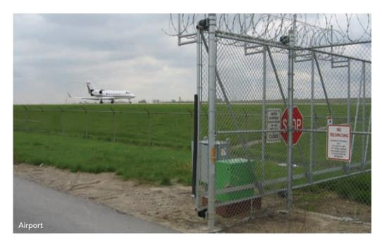
SlideDriver™ is the original ultra-reliable and secure hydraulic slide gate operator chosen for thousands of secure sites worldwide. Fully enclosed hydraulic motors drive a rigid drive rail passing between two compressed polyurethane wheels. Few moving parts. Lasts decades.
