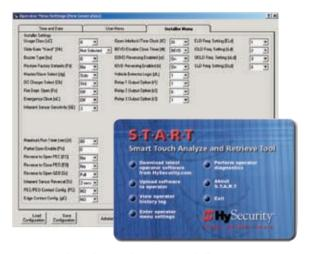
Smart Touch Analyze and Retrieve Tool allows users to upload new operator software, download fault logs, generate diagnostics, and program the operator.
