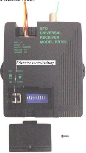
**3.** The Model RB709 will generate either a 5 second pulsed or a continuous relay output depending on the setting of the output slide switch. To energize the output relay as long as the transmitter is activated, select the CONT position. Many gate operators and some garage door openers will not work properly when the switch is in the CONT position.
