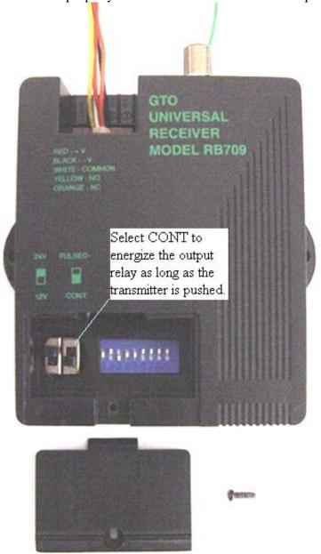
To energize the output relay for 5 seconds regardless of how long the transmitter is activated, select the PULSED position.
