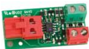
BUS XIB interface (if E024S board is used with non BUS photocells)
