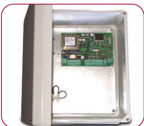
Model 455 D control panel in 10 in. x 12 in. enclosure (standard).
