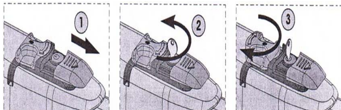
Figure 2. Use the Manual Release key to disengage the 415 Operator from its motor so that you can move the gate leaf open and/or closed by hand.
