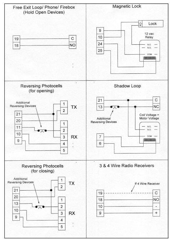
NO = Normally Open, NC = Normally Closed, C = Common, TX = Transmitter, RX = Receiver
