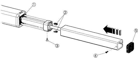
Figure 6. Install the cover for the 402 Operator
