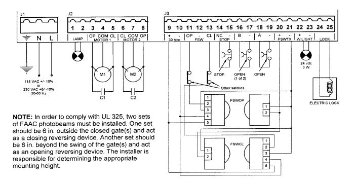
Figure 9. The terminal strip wiring of the 450 MPS
