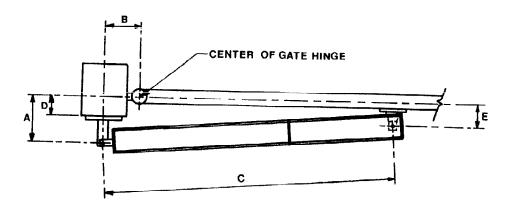
Figure 4. An inward swinging gate, top view: important mounting dimensions
