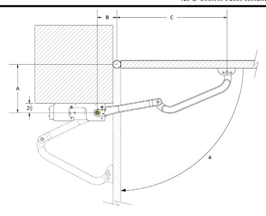
Figure 5. Dimensions for Inward Opening Typical gate applications
