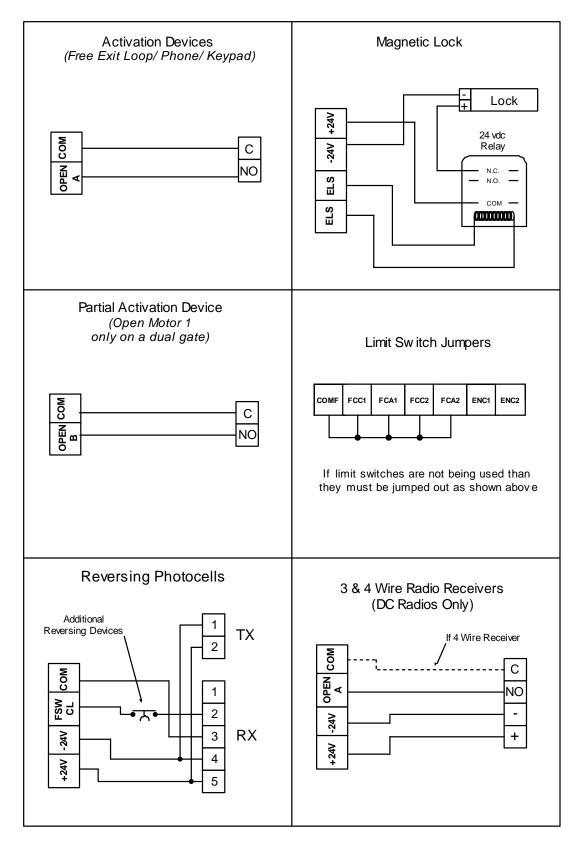
NO = Normally Open, NC = Normally Closed, C = Common, TX = Transmitter, RX = Receiver
