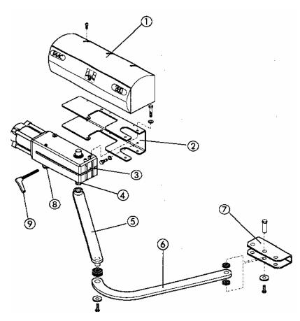
Figure 2. 390 Operator included parts.
