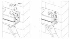
When Using 2 Limit Switches (Open and Closed Stops)
