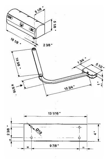
Figure 1. 390 Operator Dimensions
