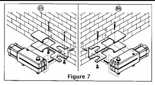
Figure 7 shows how to attach the operator to the base plate.
