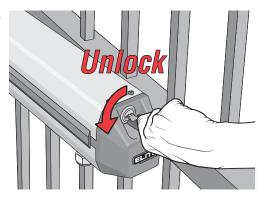
Step 2: Move the gate manually to the full open position 90°.
