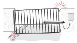
3 Gate hinges are too tight or broken and the gate is not moving freely.
