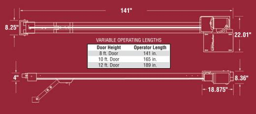
CONTINUOUS CYCLE 240 LBS. MAX. PULL COMMERCIAL DOOR AND GATE OPERATOR 1/2 HP – 120 VAC 1PH – 60HZ – 4.7 AMPS WEIGHT 123 LBS
