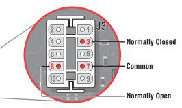
Connection of a Solenoid or Magnetic Lock can be made using the J3 plug and three wires provided with the unit.
