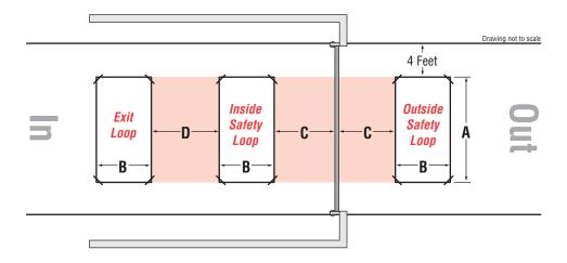
As **A** increases in size to cover a larger opening, the gate will cause a larger change of inductance when opening and closing. Therefore dimension **C** must increase as **A** increases.
