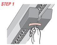
Insert key and turn to unlock position.
