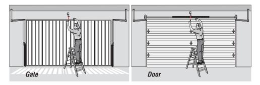
**STEP 2** Open the gate/door and mark the center point of the gate/door on the ceiling.
