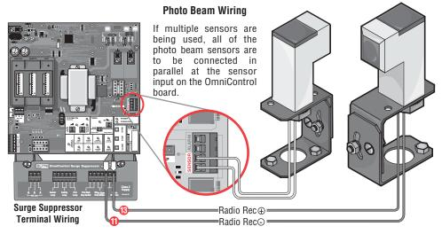
If you are going to use a non-contact sensor as a secondary entrapment protection you should use a recognized component to comply with the revised UL325 intended to be used in class I or class II gate operator, like the following:
