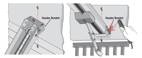
STEP 4 Lift the operator and align with center mark on ceiling. Have someone hold the operator in place or use something as a support post, and bolt to ceiling. (A support post is not part of the operator. Use only for installation.)
