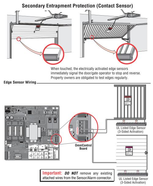
**Note:** If multiple sensors are being used, all of the edge sensors are to be connected in parallel at the sensor input on the Omni Control board.
