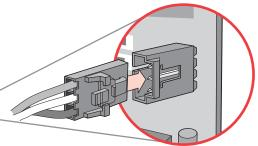
Connection of a Solenoid or Magnetic Lock can be made using the "Optional" Relay Adapter Module.
