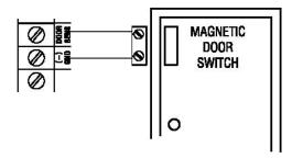
With the help of a normally closed door Position sensor (usually a magnetic door switch) on the door to set up the following functions.
