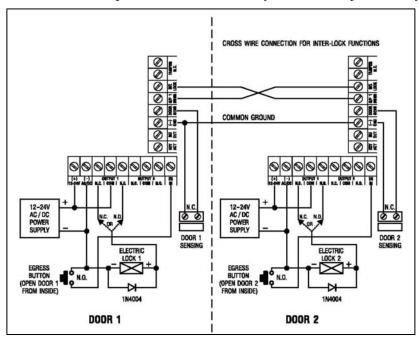
An inter-lock system needs two door controllers. This application example uses two KPX 100 with simple cross wire connection on the "Output 1 Inhibit" and "Inter-lock Control Output" terminals. It is necessary to link up the "(-) GND" terminals of the two keypads as common ground to achieve the inter-lock logic function.
