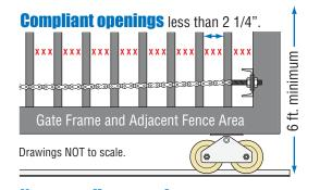
A gap, measured in the horizontal plane parallel to the roadway, between a fixed stationary object nearest the roadway (such as a gate support post) and the gate frame when the gate is in either the fully open position or the fully closed position, shall not exceed 2 1/4 inch (57.2 mm). (ref. ASTM F2200 6.1.4)
