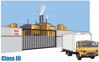
A vehicular gate operator (or system) intended for use in a industrial location or building such as a factory or loading dock area or other locations not intended to service the general public.
