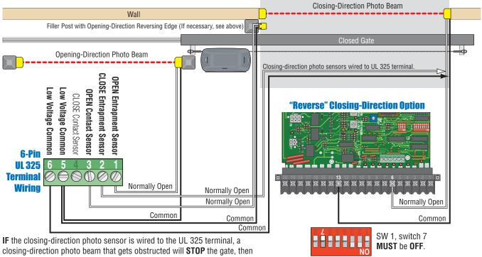
resume closing the gate when the obstructed photo beam has been cleared.
