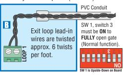
Note: The plug-in exit loop detector can be wired to partially open the gate if SW 1, switch 3 is turned **OFF**. A jumper wire must be connected from terminal #4 to terminal #5 (See next page for more information).
