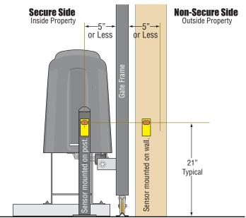
Photo sensors may be installed on either side of gate frame.
