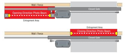
3 OPEN Contact Sensor (Reversing Edge(s)): Obstructed opening-direction reversing edge(s) will stop, then reverse the gate to the close position during the opening-direction only.
