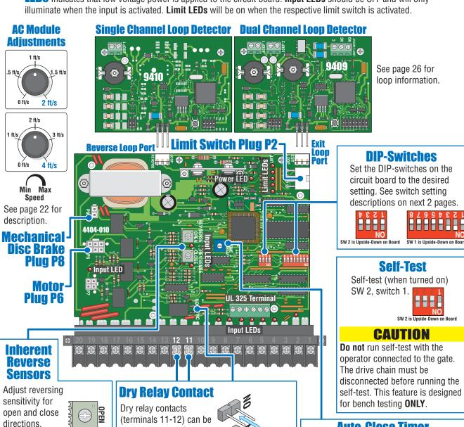
Full counter clockwise for minimum sensitivity, full clockwise for maximum
