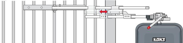
Mark and cut off excess arms. Secure arms to elbow assembly with 6 allen screws. Tighten hub and replace release tool. Install
