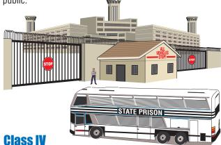
A vehicular gate operator (or system) intended for use in a guarded industrial location or building such as an airport security area or other restricted access locations not servicing the general public, in which unauthorized access is prevented via supervision by security personnel.
