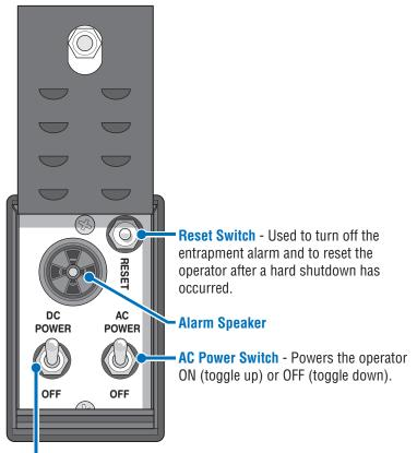
**DC Power Switch** - Turns the DC system power ON (toggle up) or OFF (toggle down).
