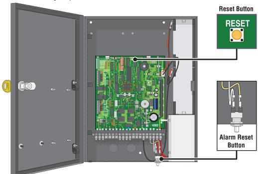
Once the gate has been reset, an open or close command is needed to start the gate operator. Most activating commands will cause the gate operator to cycle to the open position. This includes activation of a key switch or open command and activation of the automatic exit loop (If used). Activation of a close command will run the gate to the closed position.
