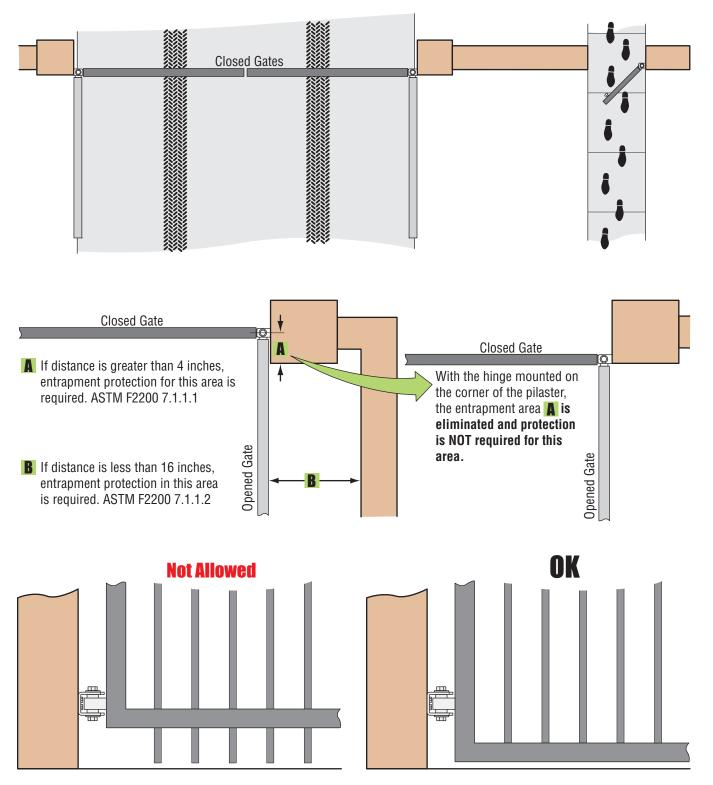
Gates shall have smooth bottom edges, with vertical bottom edged protrusions not exceeding 0.50 inches. ASTM F2200 4.3
