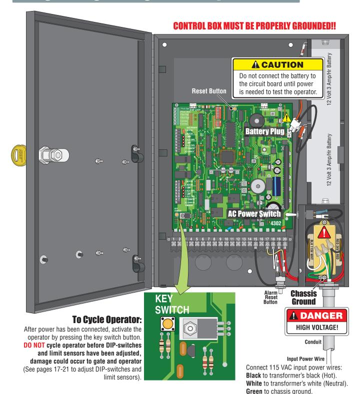
Important Power Note: To turn-off ALL power to the operator, the AC power switch must be turned off AND the battery plug must be disconnected from the circuit board.
