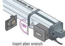
Use key to unlock and remove the cover. Remove allen wrench from inside of cover.
