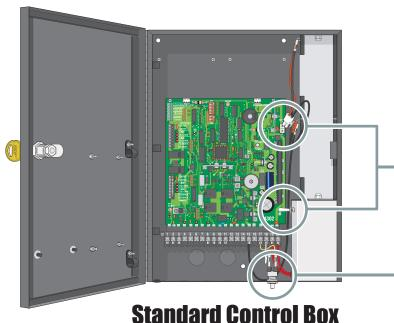
Turn OFF AC power switch AND carefully disconnect battery plug from circuit board to shut-off ALL power to operator.
