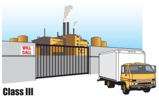
A vehicular gate operator (or system) intended for use in a industrial location or building such as a factory or loading dock area or other locations not intended to service the general public.
