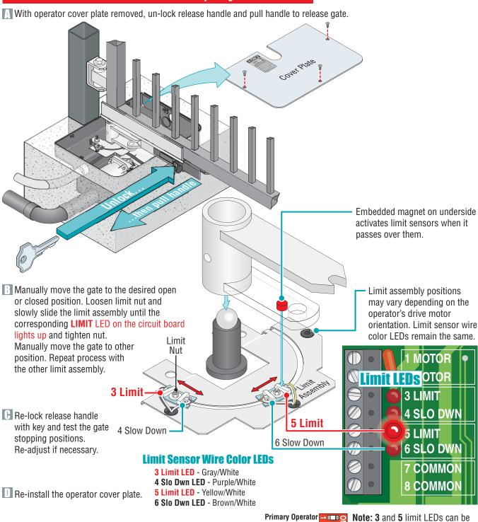
Adjust the Secondary operator limit sensors if dual operators have been installed. SW 1, switch 2 controls secondary operator opening direction. SW 1, switch 7 MUST be ON when using dual operators (See page 18).
