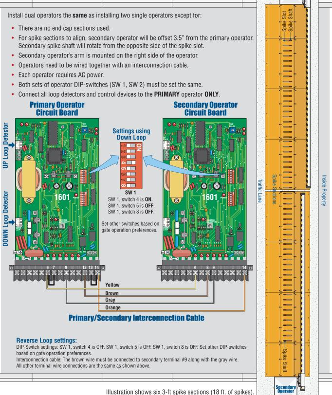
Illustration shows six 3-ft spike sections (18 ft. of spikes). Each operator controls three 3-ft spike sections.
