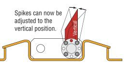
Replace the chain back into lower sprocket and tighten turnbuckle after spikes are vertical.
