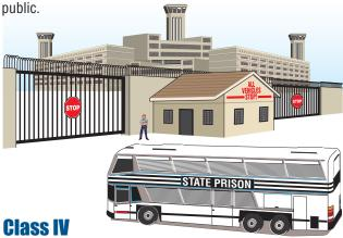
A vehicular gate operator (or system) intended for use in a guarded industrial location or building such as an airport security area or other restricted access locations not servicing the general public, in which unauthorized access is prevented via supervision by security personnel.
