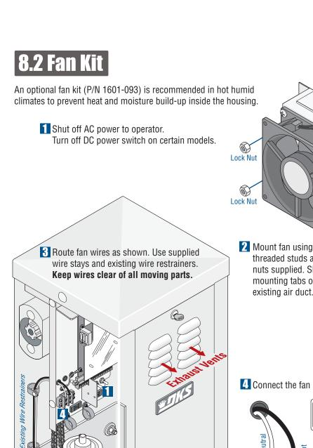
Lock Nut Threaded 2 Mount fan using 3 existing Air Duct threaded studs and lock (Existing) nuts supplied. Slide Existing mounting tabs over Air Duct existing air duct.
