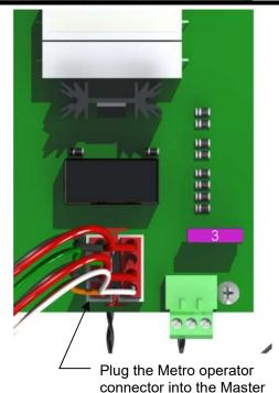
connector on the circuit
