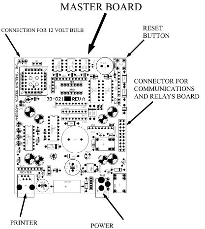
2 PIN TERMINAL WITH 2 WHITE WIRES FOR CONNECTION TO SUPPLIED TRANSFORMER
