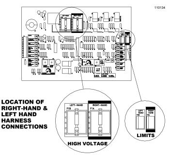
Figure 12: Right/Left Hand Control Board Connectors
