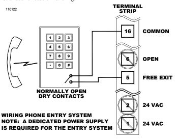
Figure 16: Wiring A Phone Entry System
