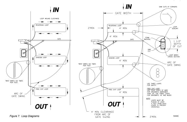
The lead-in wires need not be in PVC, but must have a least six (6) twists per running foot.
