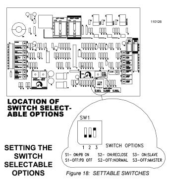
The switches that control the selectable options are located on the Control board. See Figure 18.
