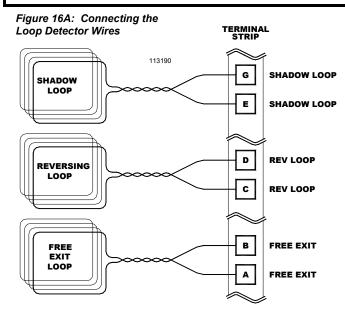
the concrete or asphalt surface in accordance with the manufacturer's instructions and the information outlined earlier in this manual (see Page 7). Connect the wires from the actual Reversing loop to Terminals C and D, see Figure 16A. If employing two (2) Reversing Loops as shown in the diagram on Page 7, and are connecting the loops to the same Loop Detector, wire in series as shown in Figure 16B
