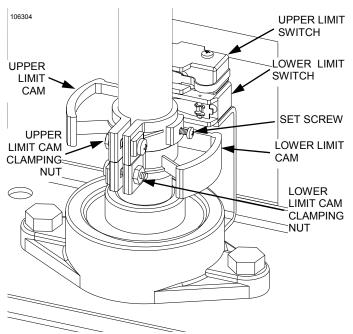
Figure 11: Limit Switches
