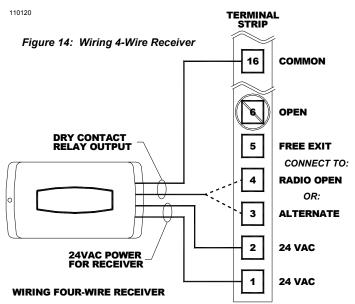
ground. See Figure 14 and the following text for proper connection.
